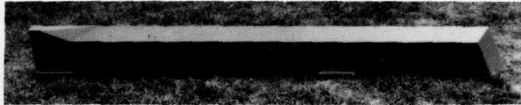
FIGURE 4* - Photograph of Simplified Sidewall With a Fairing at the Transom
