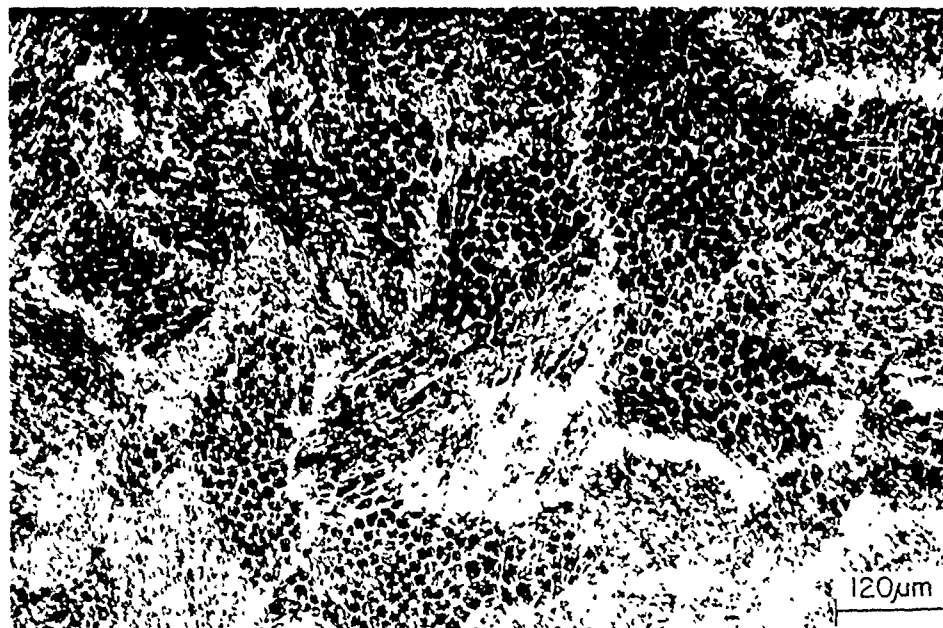
Fig. 29 — Macrostructure showing a light etched grain-boundary phase in specimen I, etched with Kalling's reagent
