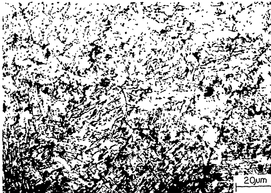
Fig. 22a — Acicular ferrite, bainite, and martensite in specimen R
