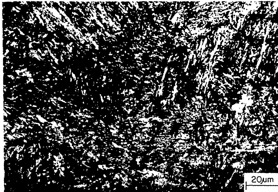
Fig. 31 — Tempered martensitic microstructure in specimen J
