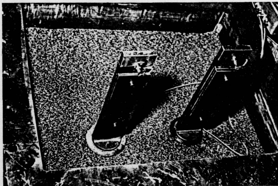
PLATE 12 - Towers on dry sand in the earthquake apparatus
