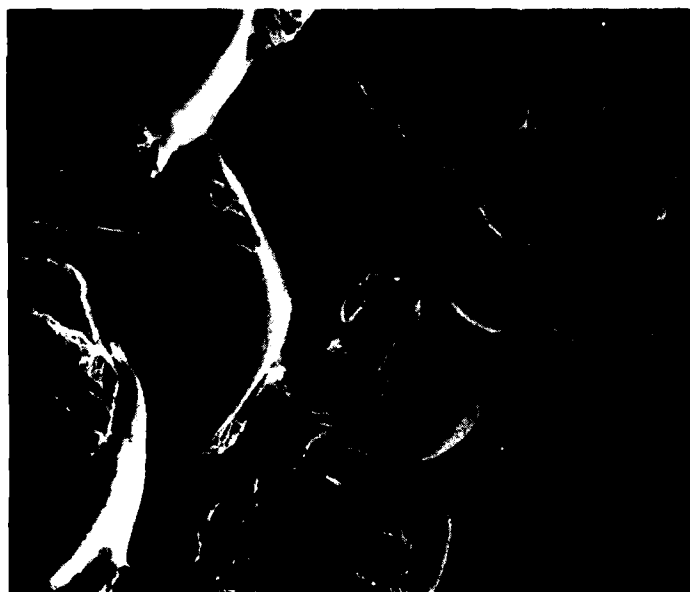
Figure 77. Microshrinkage in radius of a bond joint that failed prematurely on loading.
