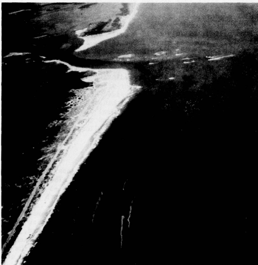
Figure 4. Aerial view of New River Inlet and the study area. Dredged sediment was placed between the two innermost dye sources. The dye pattern shows a wind-driven current moving toward the northeast.
