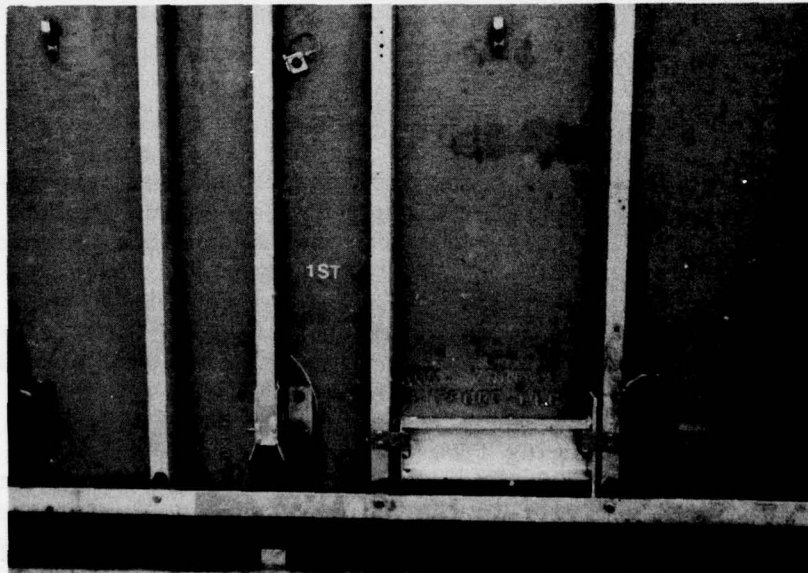
Figure 3.7.12. Auxiliary porch support legs should be taped into their brackets.
