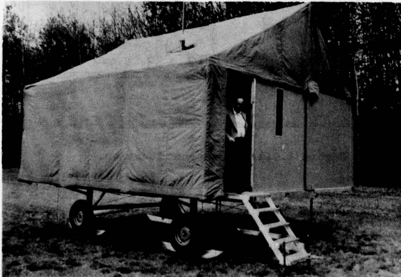
Figure 1.2.3. Tent over the shelter provides an "arctic entrance" and ample storage space.
