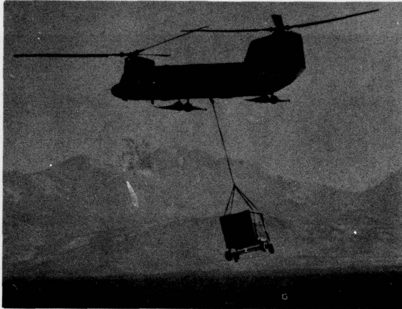
Figure 2.3.6. Rigging configuration for helicopter lift of shelter.
