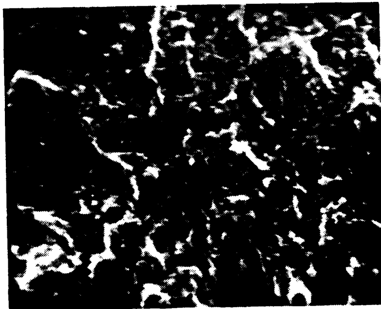
Figure 95. Higher magnification of upper area of Fig. 94 fractograph, showing lamellar secondary cracks, also characteristics of warm-rolled material. X2000.
