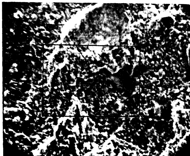
Figure 31. SEM fractograph of Fig. 30, in the fatigue zone, showing transgranular fracture and many secondary cracks. X1200.
