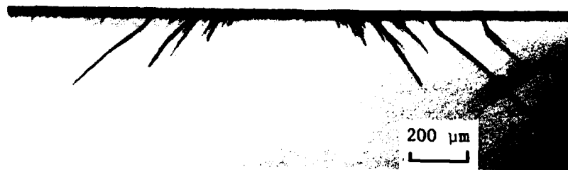
(b) Shot no. 1215: 1.96 mm nylon bead at 381 \text{ ms}^{-1} .
