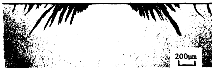
(c) Shot no. 1200: water drop impact at 354 \text{ ms}^{-1} .
