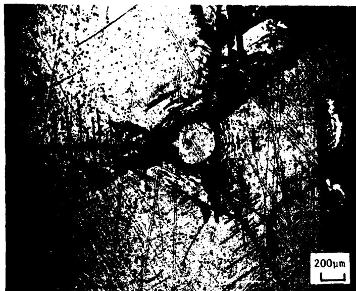
Figure 3.21. Etched water drop impacted surface of (111) \text{CaF}_2 . Impact velocity is 520 \text{ ms}^{-1} . Arrows indicate cross section shown in Fig. 3.23a.
