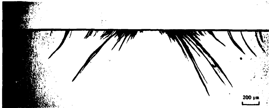
(e) Shot no. 1235: water drop impact at 540 \text{ ms}^{-1} .
