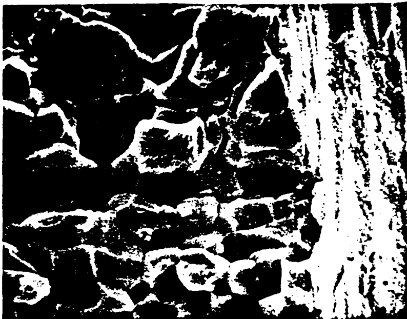
Figure 22. Region of intergranular fracture at edge of alloy B thermal specimen. Note that secondary cracks are also intergranular (1000 X).
