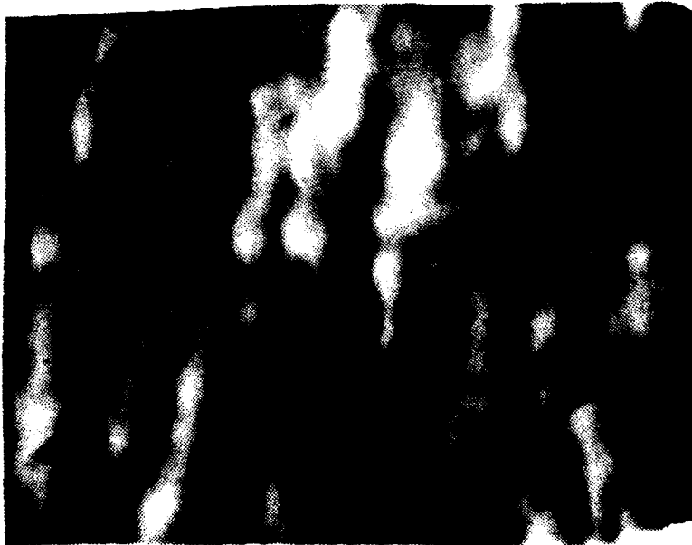
(d) Speckle size imaged by lens of f/5.6
