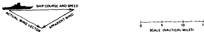
FIG 5.4 APPARENT WIND VECTOR RELATIONSHIP TO THE ACTUAL WIND AND THE SHIPS COURSE AND SPEED
