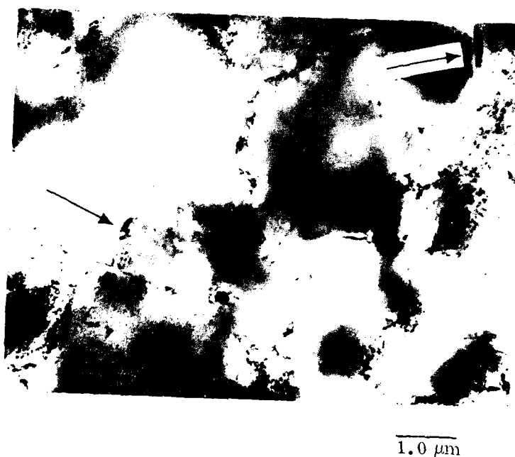
Figure 8. Subgrain structure in Alloy 1.2 (Al-3Li-2Cu-0.2Zr) (TEM).
