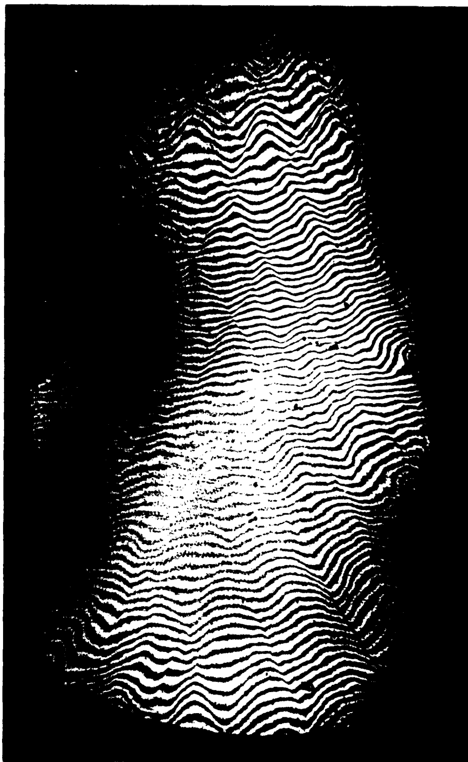
FIGURE C-10. DOUBLE PULSE LASER HOLOGRAPHY OFFSET FRINGE (RUN 45, t = 188 \mu\text{SEC} ).
