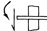
C. NON-SYMMETRICAL FLEXURAL-SHEAR FAILURE DUE TO LATERAL LOADING.
