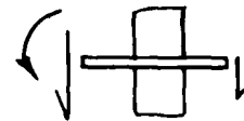
B. NON-SYMMETRICAL FLEXURAL-SHEAR FAILURE DUE TO EITHER NON-SYMMETRICAL LOAD PATTERN OR TO FAILURE OF AN ADJACENT JOINT
