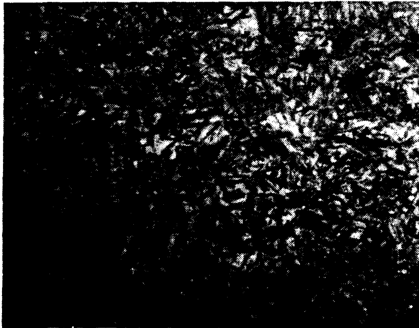
Figure 21. Micrograph Of 550 C Rolled 52100 After Treatment 250-IT. Microstructure consists of bainite and martensite. 1000X
