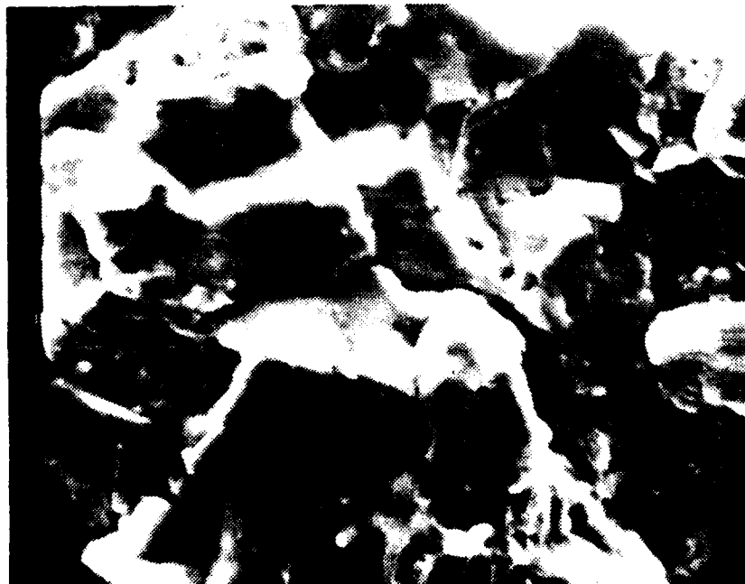
Figure 32. Fractograph Of Standard 52100 Fracture Surface After Hardening Treatment 850-ST. The flat surfaces are clear evidence of brittle fracture. 2000X
