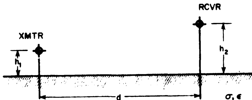
Figure B-1 Geometric parameters used to calculate the non-directional beacon field strength.
