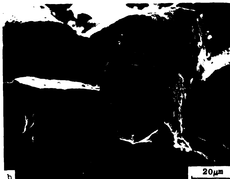
Fig. 8 — Scanning electron micrographs of intergranular cavities associated with precipitates in annealed Type 316 stainless steel irradiated to 4.8 \times 10^{22} \text{ n/cm}^2 at 649^\circ\text{C} and tested with a two-minute hold time at 649^\circ\text{C} .
