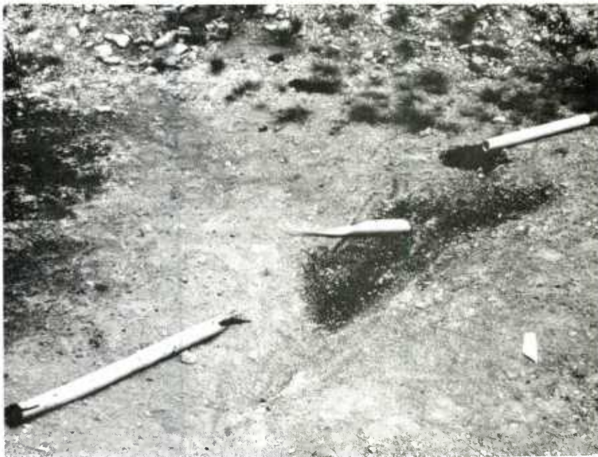
Figure 13. Typical PVC feed pipe fragments, IMR 8208 propellant test series
