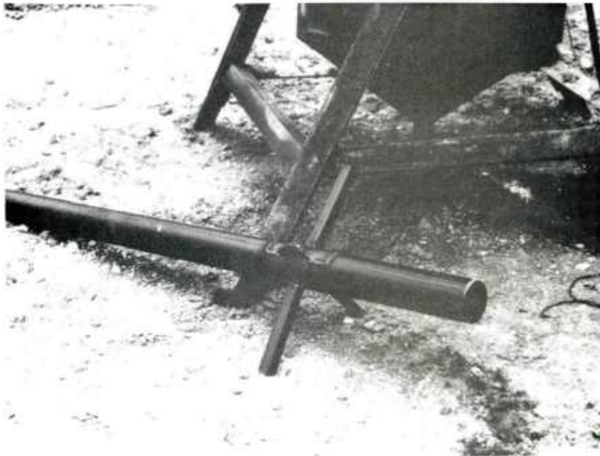
Figure 23. "Vent pipe" of SCAMP hopper after 91 kg of WC 844 propellant were initiated in hopper
