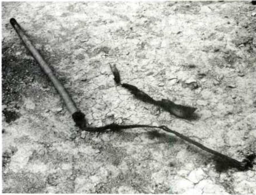
Figure 12. Steel feed pipe and fragments after explosion reaction of IMR 8208 propellant within the pipe
