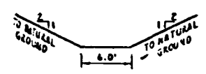
TYPICAL SECTION OF OUTLET CHANNEL EXCAVATION EXIT CHANNEL EXCAVATION EQUALS OR EXCEEDS DESIGN SECTION. SEE "CROSS SECTIONS FOR PAYMENT"
