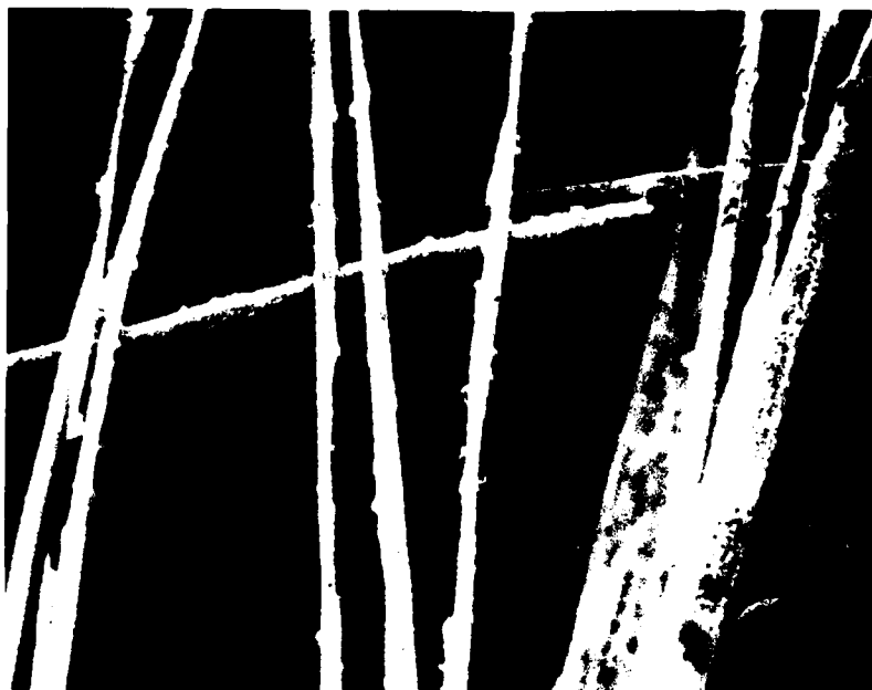
Figure 16. Section of fiber remains from bottom 2 plies of Hercules AS/3501-6 (resin modified with Pb_3O_4 ) after self-sustaining combustion test; Air flow = 8.3 mph (SEM photomicrograph, 1000 X magnification)
