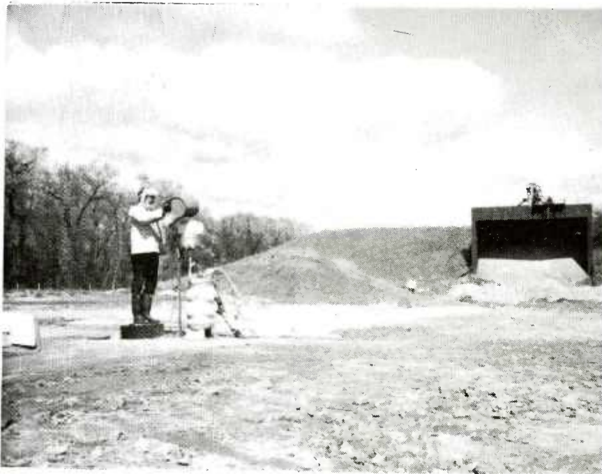
Fig D.10 Pouring liquid DNT into the drop tank
