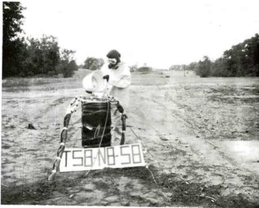
Fig D.9 Pouring liquid TNT into tank
