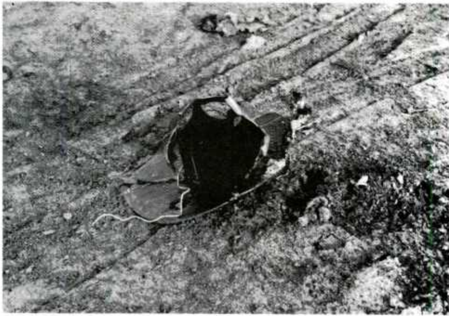
Fig D.23 Nitrator 8 cover and draft tube assembly remains (90.8 kg (200 lb) of TNT at NSTL)
