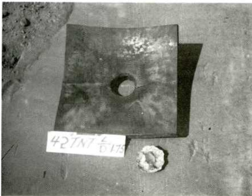
Fig D.18 TNT cylinder witness plate damage
