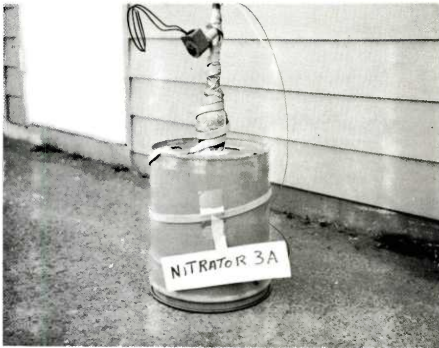
Fig D.5 DNT drop-in tank and solenoid (upside down)
