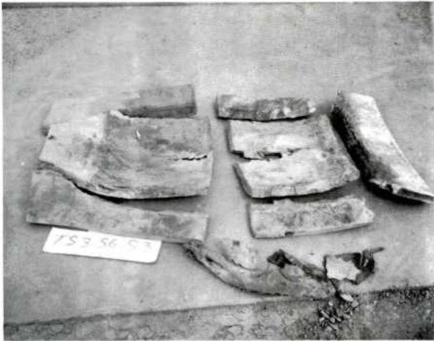
Fig D.15 Witness plate damage for separator detonation
