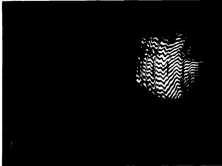
Fig. 2.2. Secondary Mirror. This represents the surface prior to polishing using the Parent system test.
