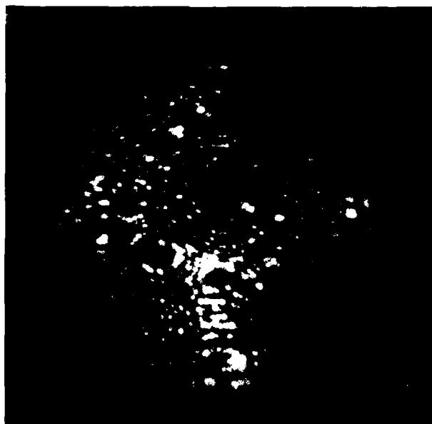
Figure 10 A helium-neon field ion micrograph obtained from vanadium preimaged with hydrogen, 12 kV, 30 K.
