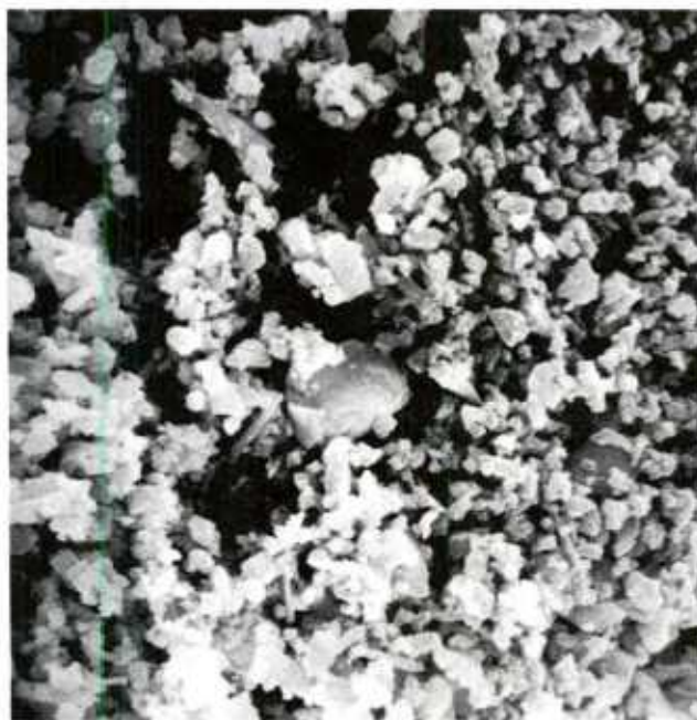
Figure 3. Typical SEM photomicrograph of the \text{Si}_3\text{N}_4 particles of processed Sylvania powder of batch SN502-87. Mag = 5000X.
