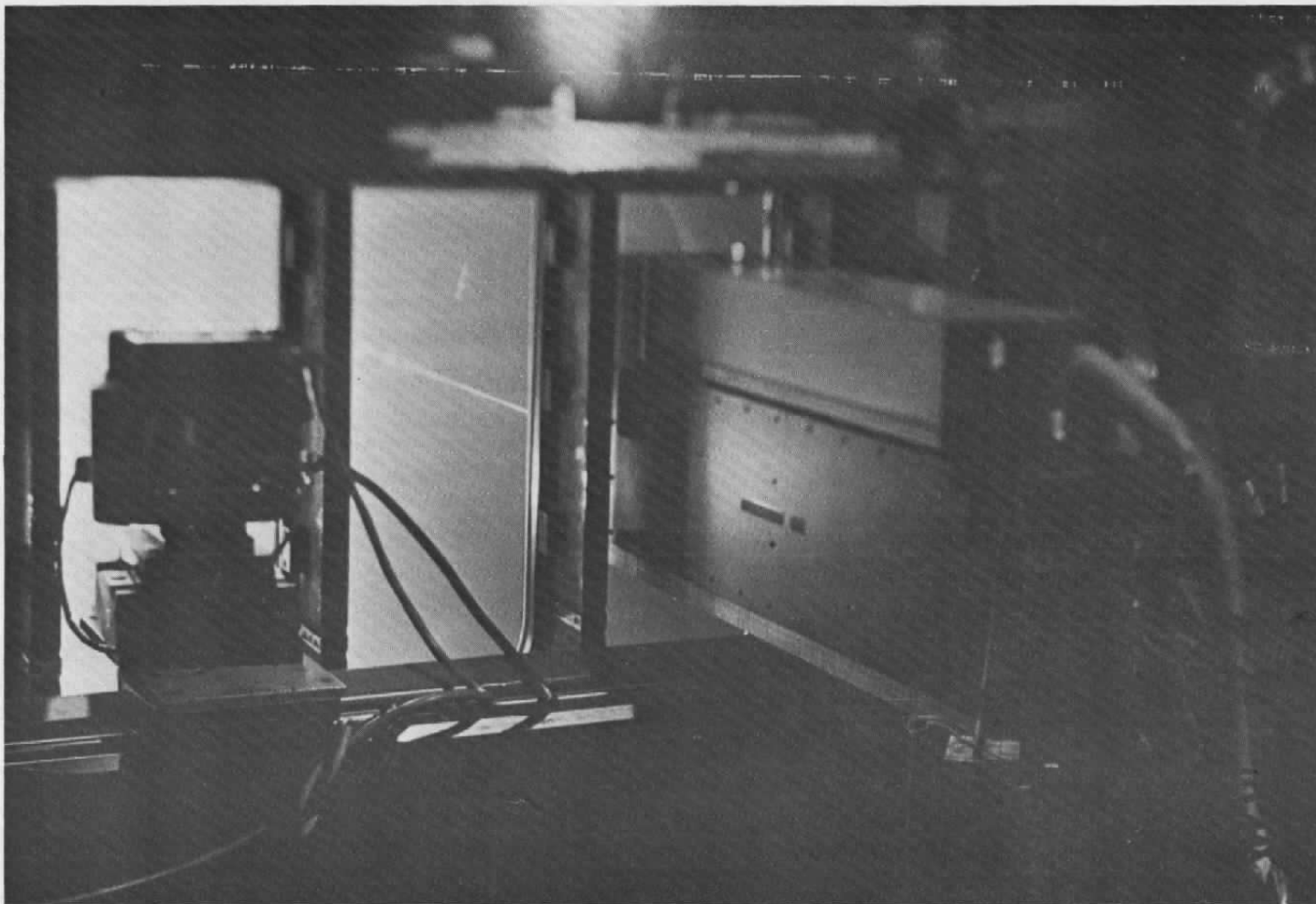
Figure 22. Optical Head with Beams Entering Fog in Tunnel A.
