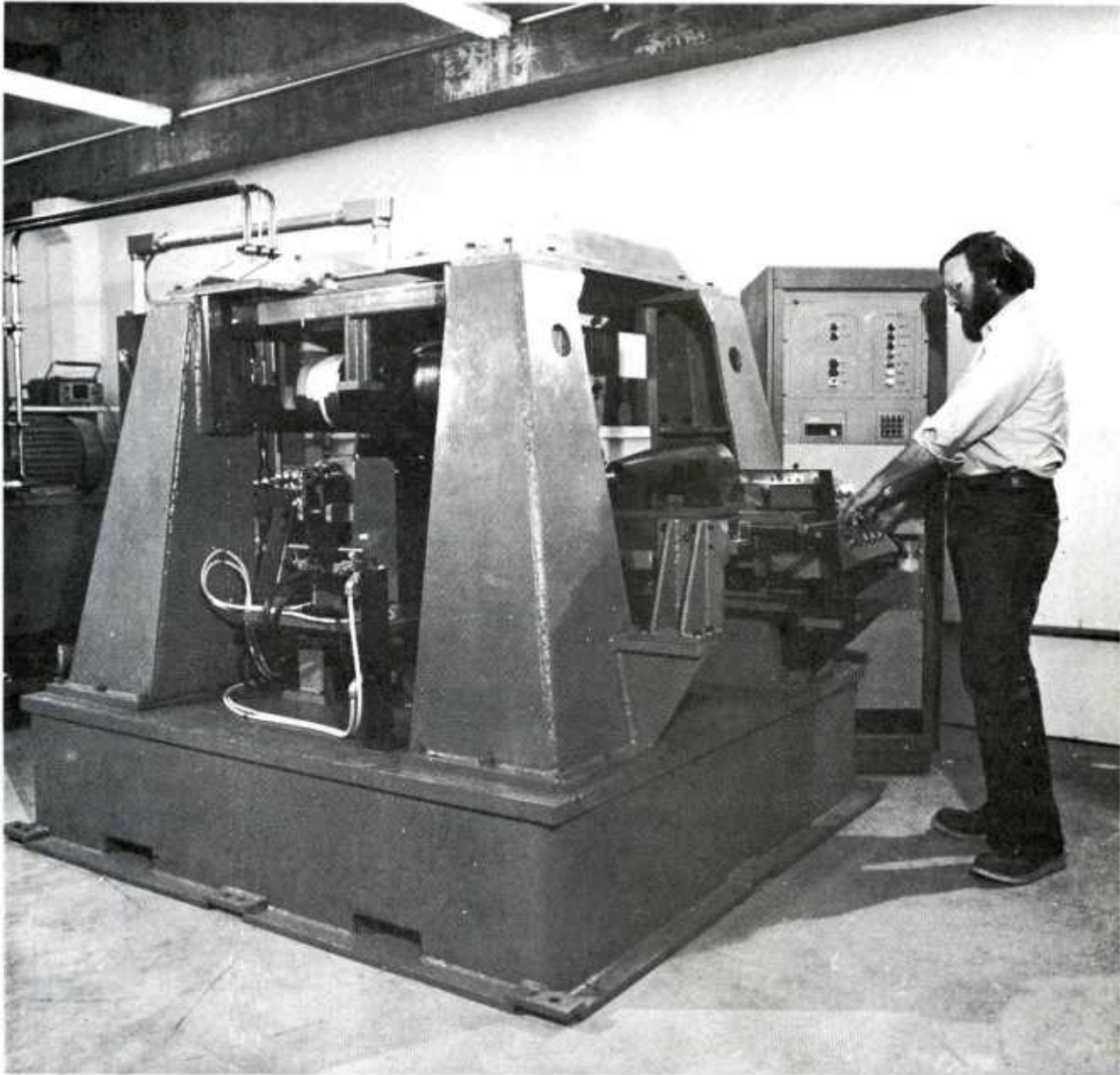
Fig. 51 Photograph of fully assembled EMAT inspection system during projectile inspection.
