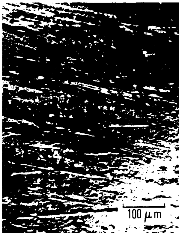
Fig. 11. Nomarski View of Mirror with Heavy Blue Haze After Incomplete Film Removal by Rubbing in Cold Water
