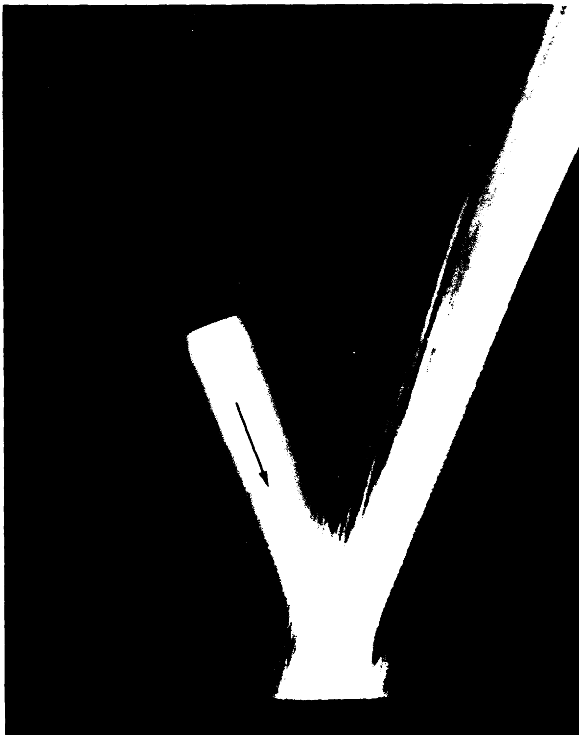
Figure 1. Schlieren photograph of an ultrasonic beam of Gaussian cross section reflected from a brass grating in water.
