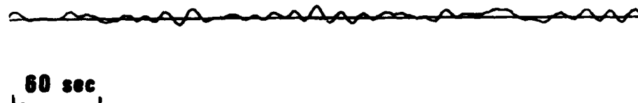
Figure 3. Records of noise from the four NSS recording channels and from the SDCS SP and LP seismographs. Part of the noise sample No. 27 (ref. App. 1) is shown.
