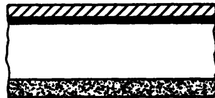
Category B Inner Surface Corrosion
