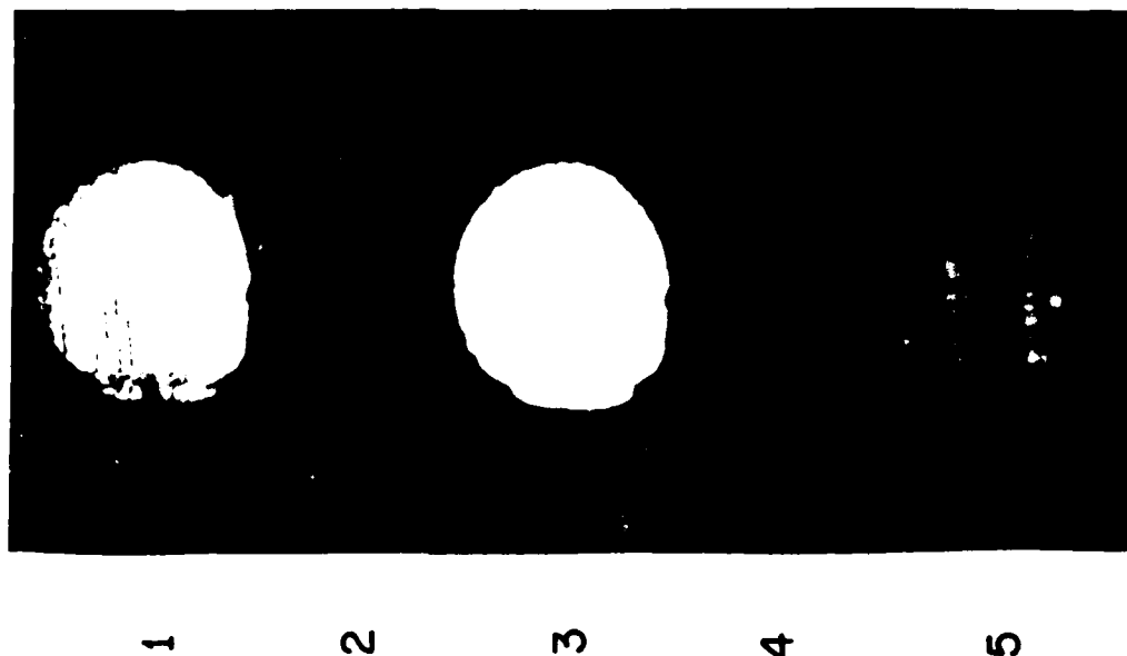
FIG. 8 IMAGE CONVERTER INTERFEROGRAMS OF A TRAVELLING SHOCK WAVE IN ARGON USING A RUBY LASER IN NORMAL-LASING MODE AS A LIGHT SOURCE.
