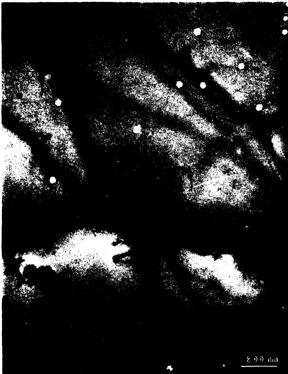
Fig. 2 — Ni-1% Al at 675 C. This area is typical in both void size and density
