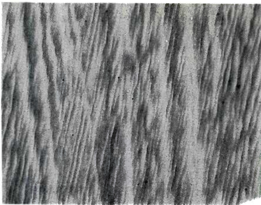
FIG. 20a - 0323 - OD 20X - Residual Dendritic Structure (Normalized)
