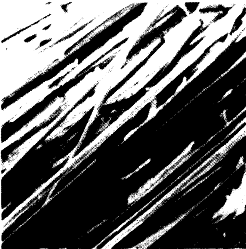
FIGURE 3. SEM Tensile Fractographs of Failure Surfaces in Al/Gr Composite. Tensile Loading Axis Parallel (A, B) and Perpendicular (C, D) to the Fiber Reinforcement Direction.
