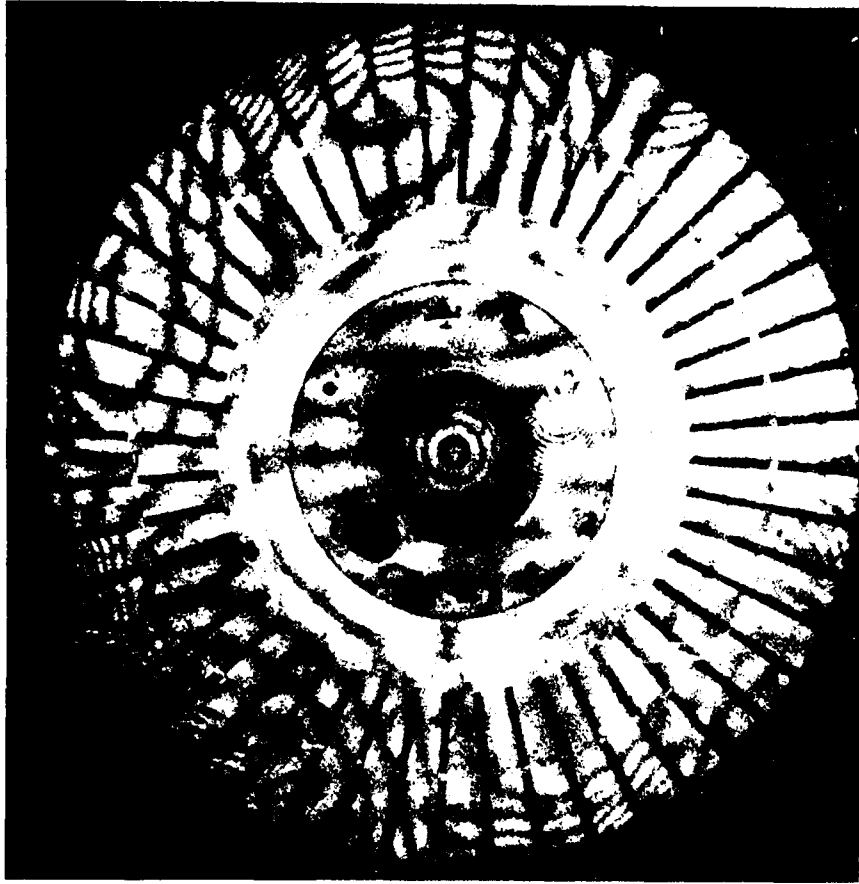
Figure 28. Image Derotated Double Exposure Hologram of the 3N-1S Mode of Vibration of the J52 2nd-Stage Compressor Bladed-Disk Rotating at 7500 rpm (the Excitation Frequency was 300 Hz and the Response Frequency was 670 Hz)
