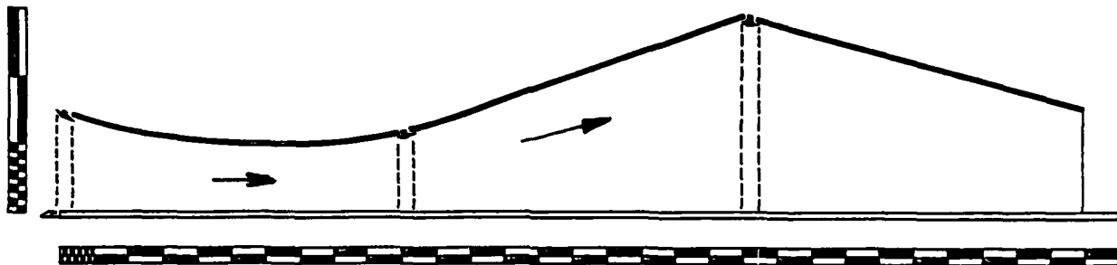
FIGURE 1. SIDEVIEW SCHEMATIC OF THE TEST SECTION. MAJOR DIVISIONS ON SCALES: 10 INCHES. NOTE BAFFLE PLATE UPSTREAM OF BLUNT LEADING EDGE ON BOTTOM TEST WALL AND SIDE AND UPPER WALL JET BOUNDARY LAYER CONTROLS.
