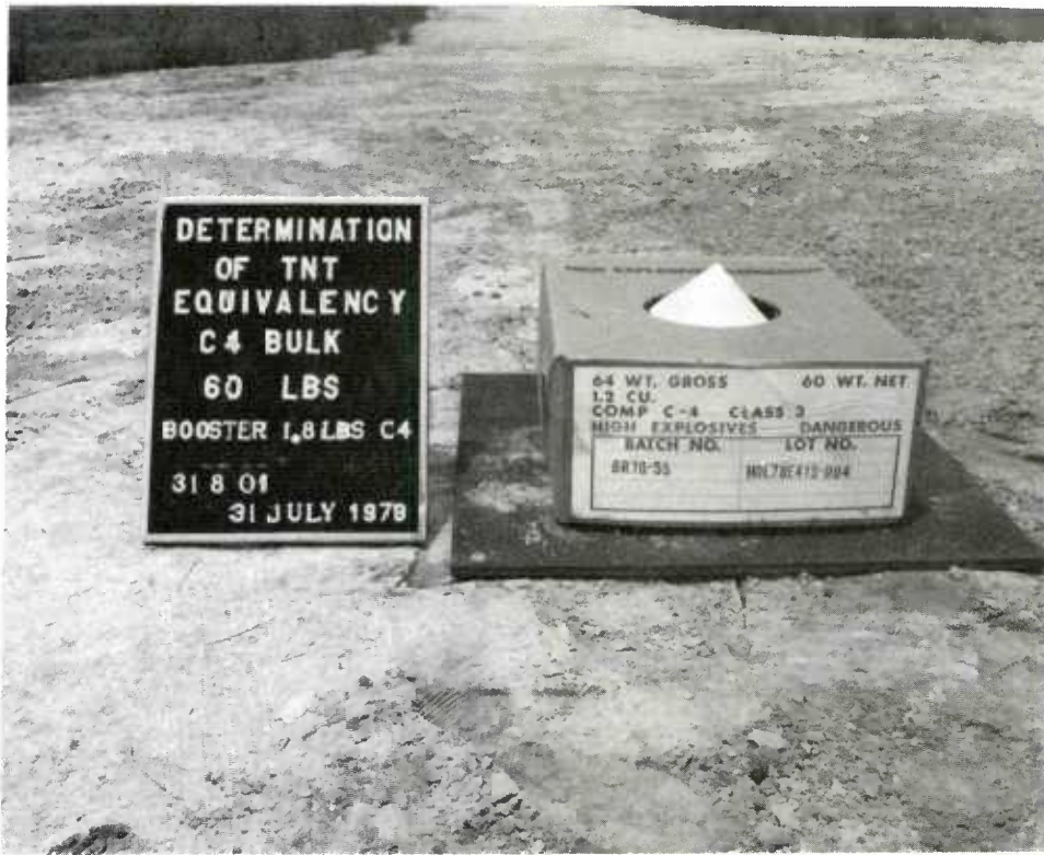
Pretest Configuration 27.2-kg Charge
