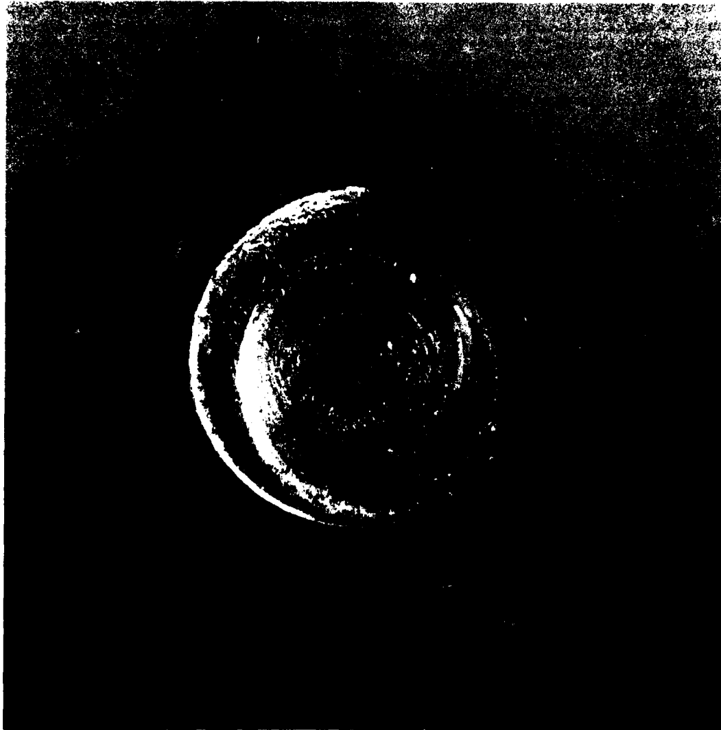
Figure 1. Eccentric Roller End Wear Due to Interaction With the Face of the Inner Ring Guide Flange
