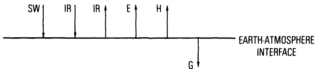
Fig. 2. Energy Balance at Earth-Atmosphere Interface
