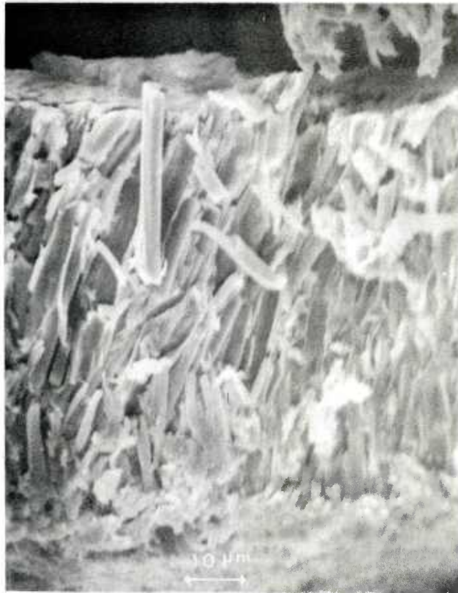
Figure B-3. SEM of M30A1 propellant lot E2 at 1000X magnification and 20 KV
