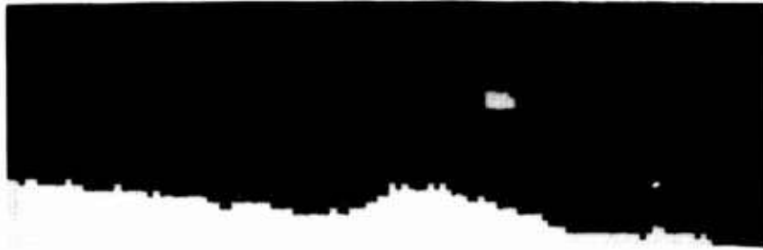
MOISTURE DISTRIBUTION IMAGE - LIGHTER SHADE INDICATES HIGHER MOISTURE CONTENT
