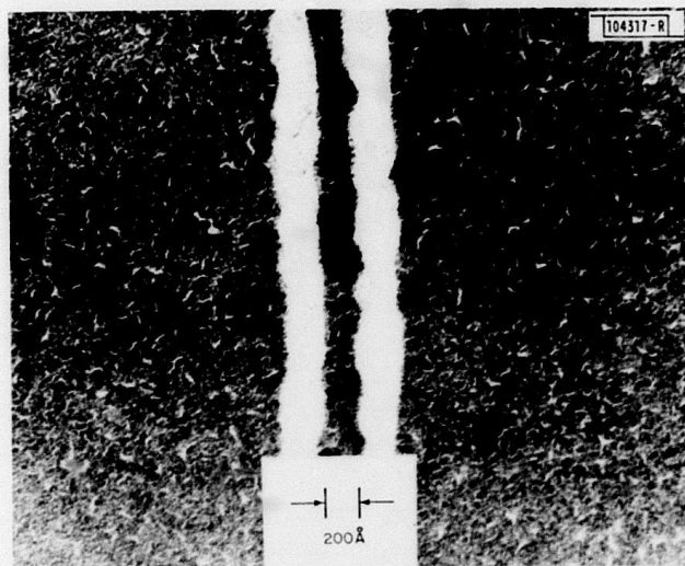
Fig. 6. TEM of a 50-Å-thick electrically continuous tungsten pattern on a SiO 2 substrate produced by liftoff using a PMMA pattern similar to that shown in Fig. 5. Tungsten was evaporated onto the structure at normal incidence and the PMMA was dissolved in monochlorobenzene.
