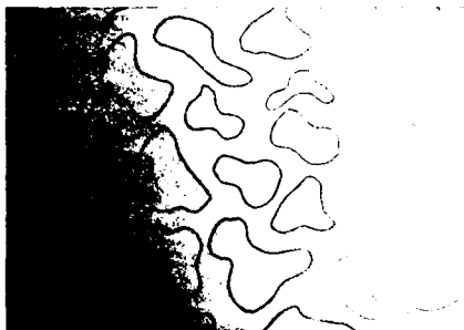
Fig. 40 — The advanced stage of castor-oil permeation with diffusion through the rubber matrix as the controlling factor
