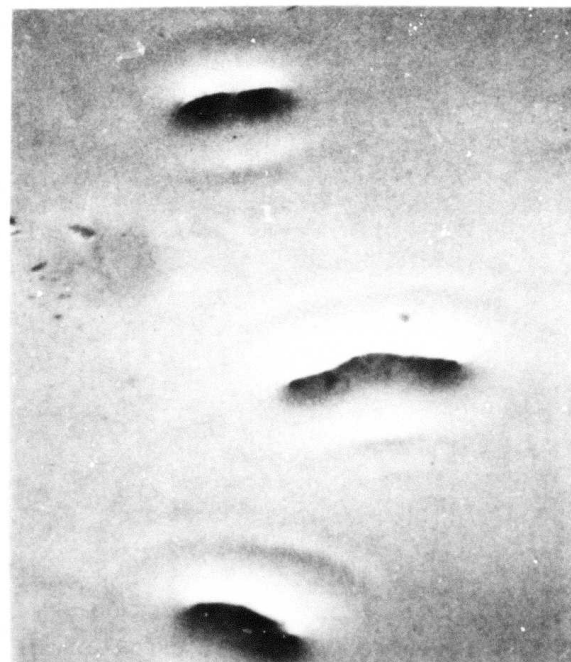
FIG. 7. Scanning electron micrograph of neutron irradiated silicon surface exposed to a ruby laser pulse of 2.0 J cm -2 , magnification 3000 \times .
