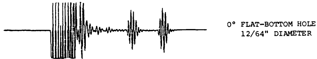
FIGURE 4.6: EXAMPLES OF PULSE-ECHO RECORDINGS OBTAINED FROM THE INBOARD ARRAY
