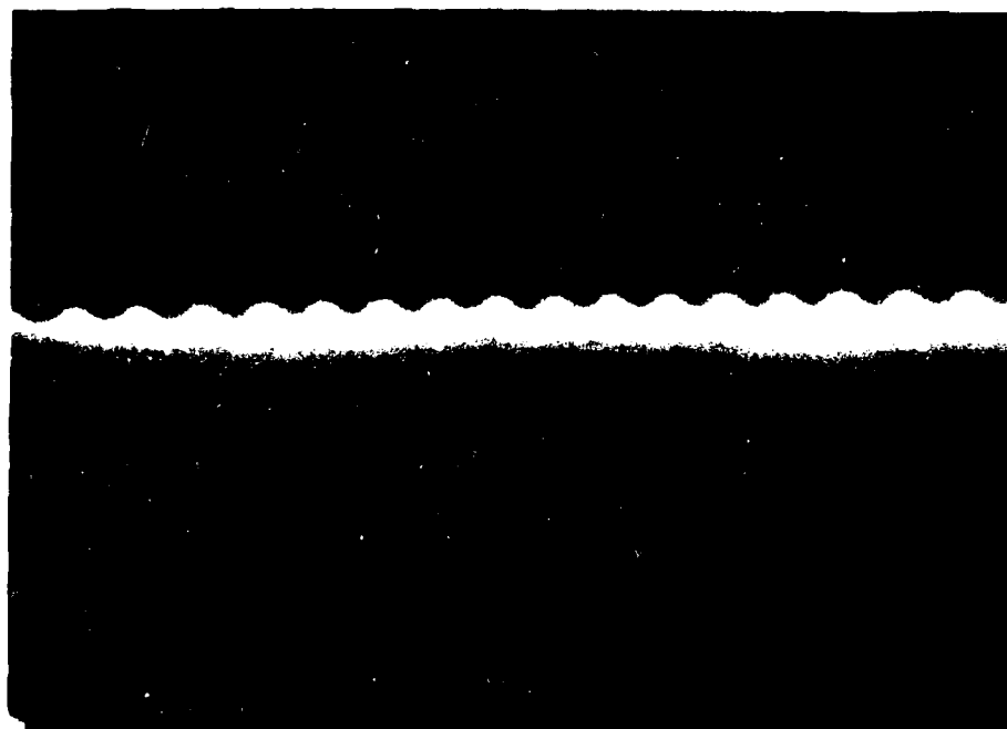
Fig. 4-20. Cross Section Through Ion-Milled DBR Reflector. Grating periodicity is 3600 Å.
