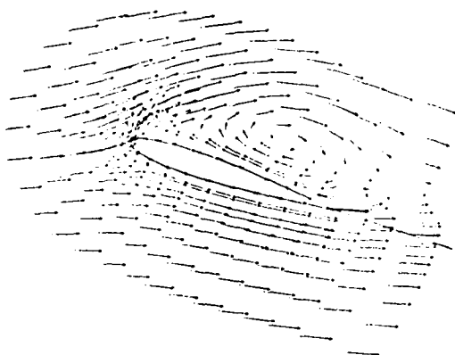
Figure 10. - Computed velocity vector field, \alpha = 19^\circ , t = t_1 .
