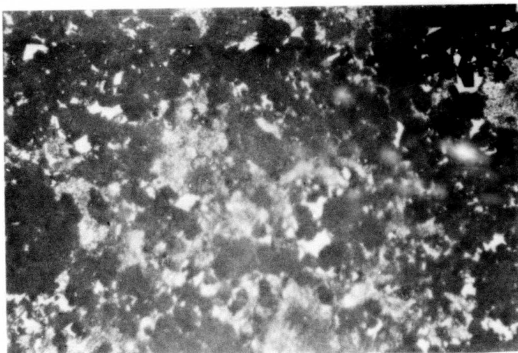
Figure 8. Duplex Structure at the Edge of a Coarse-pored Siliconized Sample.
