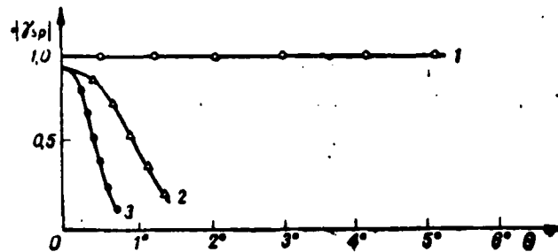
Fig. 2. Dependence of the modulus of spatial coherence function on angular distance between points.
