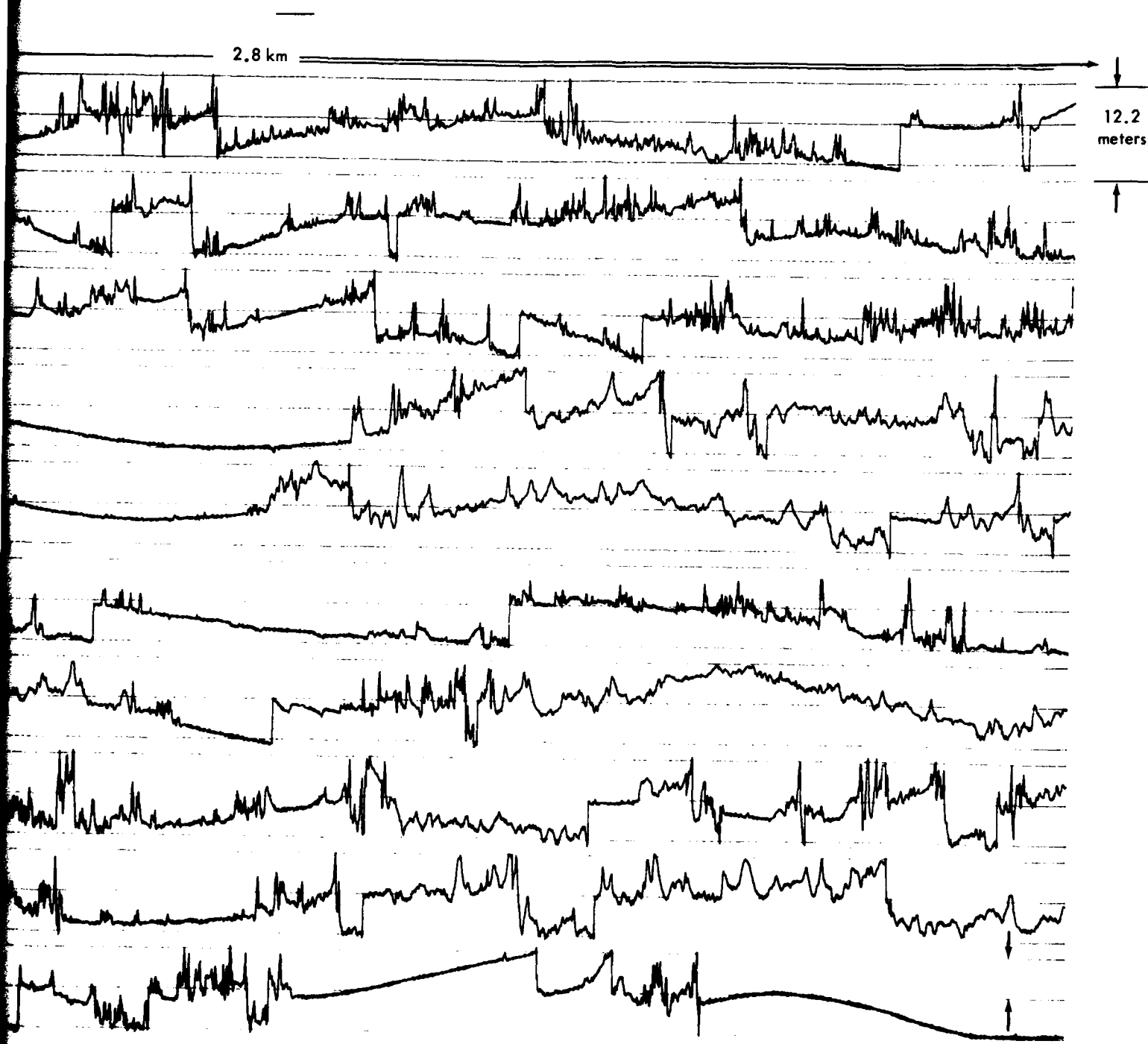
3. Laser sea-ice profile with many discontinuities. Circled area is one of several in which two or three discontinuities occur in rapid succession.
